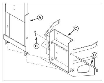
Figure 4. Install Back Plate (Flat Style Bumper shown)
